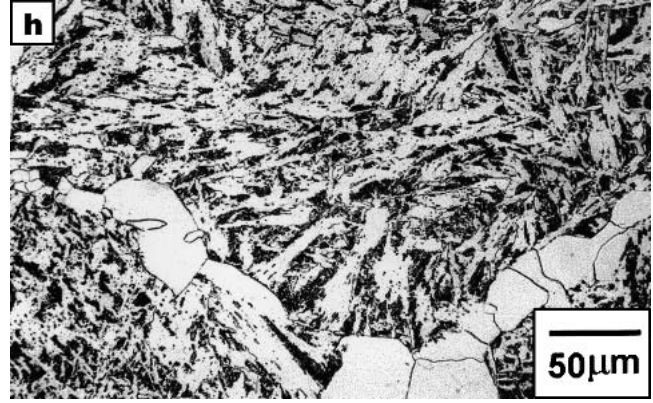
Fig. 2 cont. (a) Schematic drawing of annealing routes applied to the original A508 steel (A); and (b) light micrographs of embrittled microstructures B (c) C, (d) D, (e) E, (f) F, (g) G, and (h) H (nital etch)
